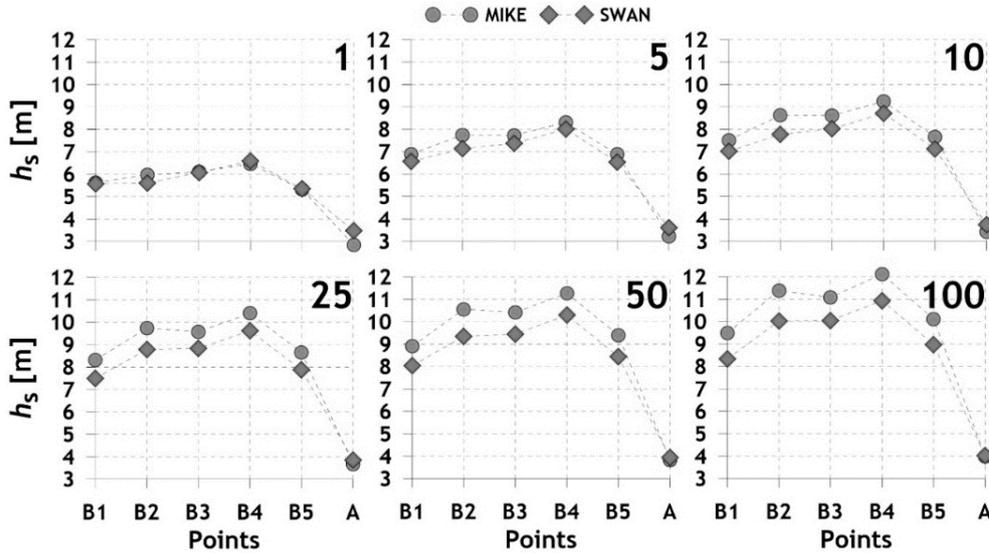
**Fig. 6:** Significant wave heights, possible once in a given number of years, at selected points of the area.
