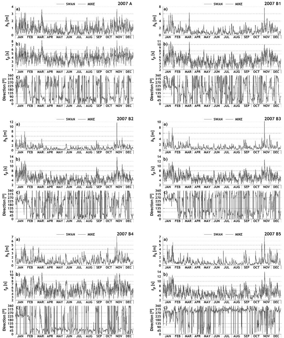
**Fig. 2:** The series of significant waves heights (a), the periods of the peaks of the spectrum (b) and the directions of propagation of the waves (c), obtained by calculation at given points.
