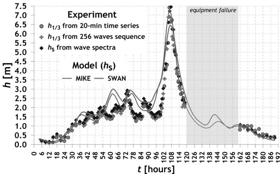
**Fig. 4:** Comparison of experimental and model wave heights in an extreme storm.
