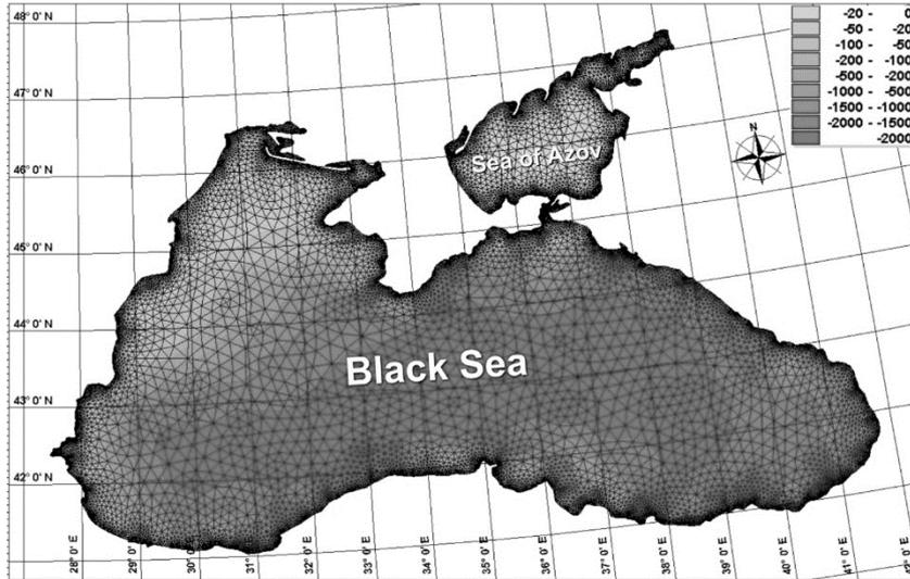
**Fig. 1:** Bathymetric map (m) and computational grid for the Black and Azov Seas area.
