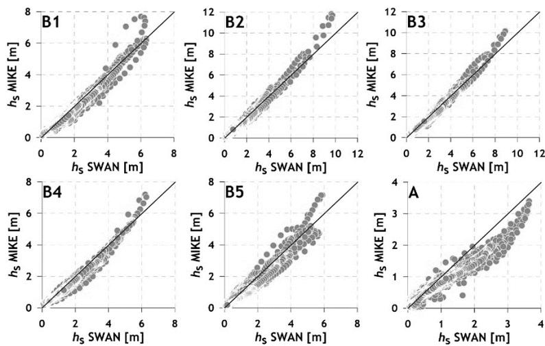
**Fig. 3:** The ratio of significant wave heights obtained by the two models at selected points (data for 2007).
