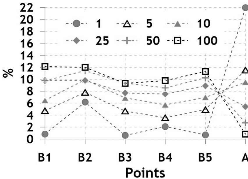
**Fig. 7:** The difference (in percent) between the values of significant wave heights, possible once in a given number of years, obtained by the models MIKE and SWAN.
